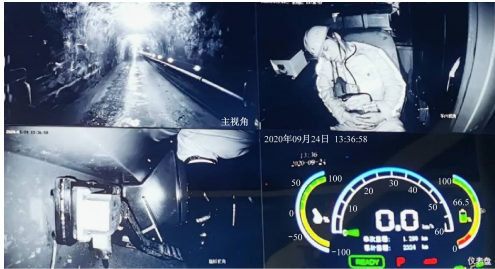
图4 智能辅助运输视频监控画面 Fig. 4 Video monitoring screen of intelligent auxiliary transport
