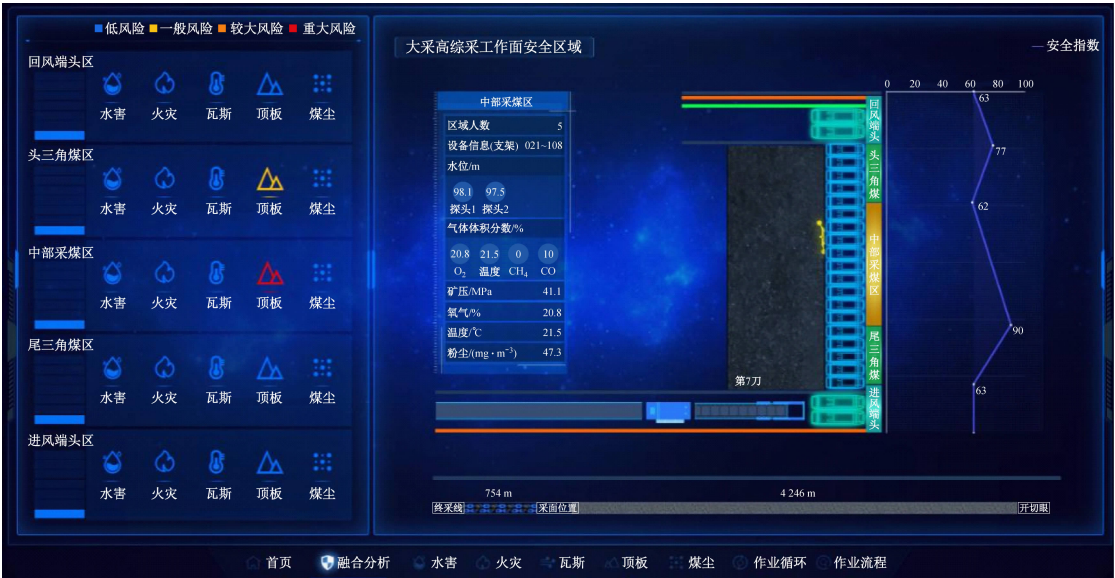
图 2 大采高综采工作面环境安全监测分析界面 Fig. 2 Interface for environment safety monitoring and analysis of fully-mechanized working face with large mining height
